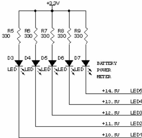
Fig. 7 Battery voltages monitor display
