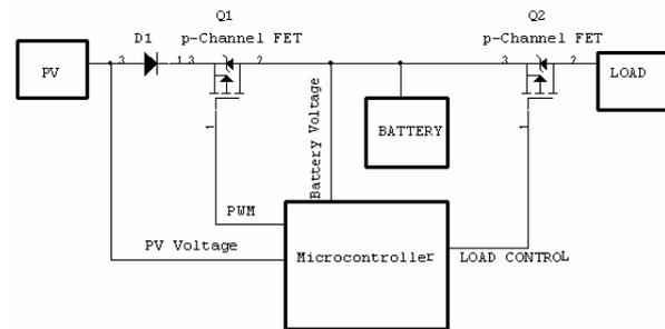
Fig. 2 Block diagram of charge controller
