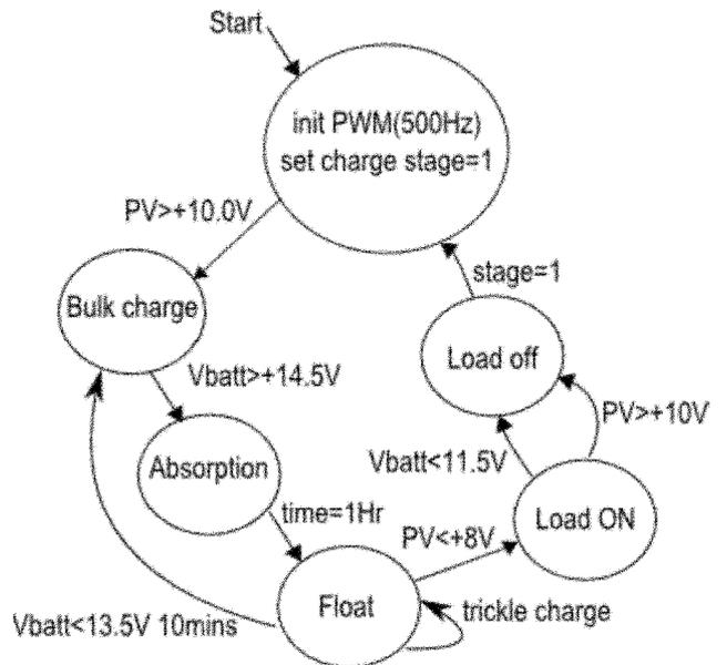
Fig. 10 State diagram of the main loop
