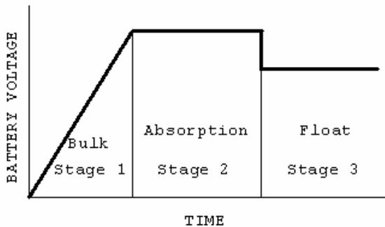
Fig. 1 Three stages charging profile
