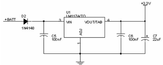
Fig. 9 Power supply circuit
