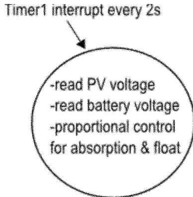
Fig. 11 Functions serviced by timer1 interrupt
